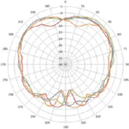
**Elevation plane (side view, 90 degrees angle)**
